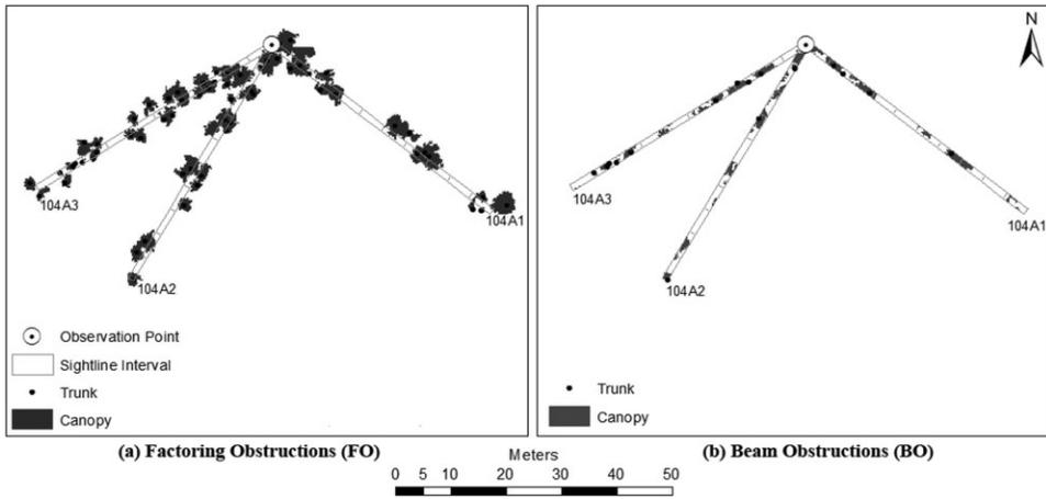
**Figure 2** Comparison of trunk and canopy extraction for plot 104A: (a) Canopies and subsequent trunks intersecting the 1 m<sup>2</sup> wide sightline beam were selected as factoring obstructions (FO); and (b) Vegetation instances inside the beam were quantified as beam obstructions (BO)
