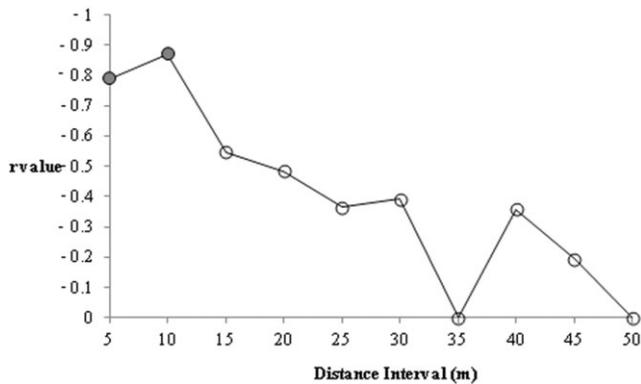
**Figure 3** Spearman rank correlation (r) between TLS and reference visibility at 5 m distance intervals (n = 12). Values at 5 and 10 m (grey circles) were significant (p = 0.05)
