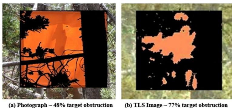
**Figure 4** Obstruction comparison between digital photography and TLS imagery of 1 m<sup>2</sup> target in plot 104A1 at 10 m: (a) High resolution of digital photography enables delineation of branch and needle obstructions (trunk and branches are colored black in image); and (b) TLS data produces a coarser representation of obstructions
